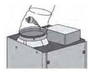
5. Remove the grease mesh filter and install active charcoal filter (Not Supplied) onto motor chamber refer below drawing.
