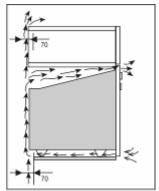
The unit panels next to the appliance must be heat resistant. In the case of veneered wood units, glues must be resistant to a temperature of 120°C.
