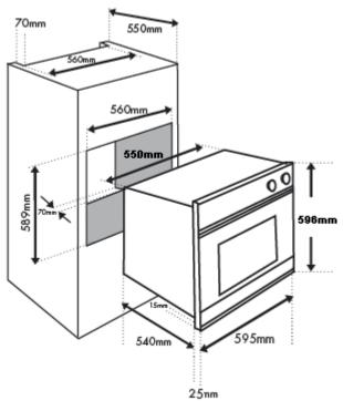
To provide adequate ventilation, there must be appropriate ventilation opening, the panel to which the oven is fitted should have a gap of at least 70 mm at the rear.
