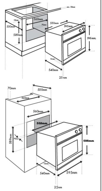
To provide adequate ventilation, there must be appropriate ventilation opening, the panel to which the oven is fitted should have a gap of at least 70 mm at the rear.
