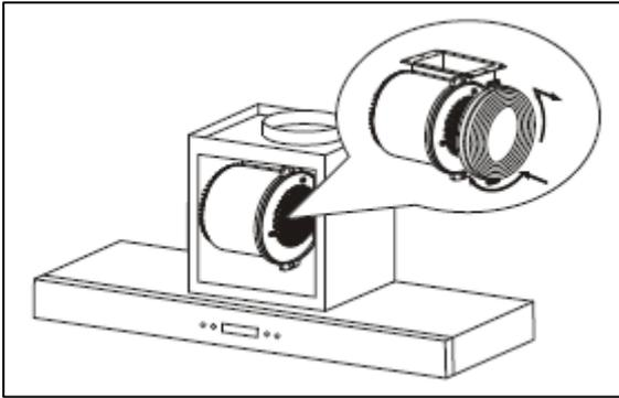
4) Hook the carbon filter over the pins that are located at the end of the motor.
