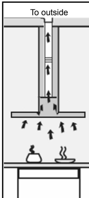
For air extraction mode, a ducting kit is required, the air is drawn in and cleaned by the grease filters and via the ducting must be directed to the outside atmosphere.
