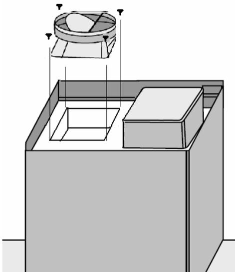
5. Fit the *flexible exhaust duct* onto *outlet*. ( *Air Extraction mode only* )
