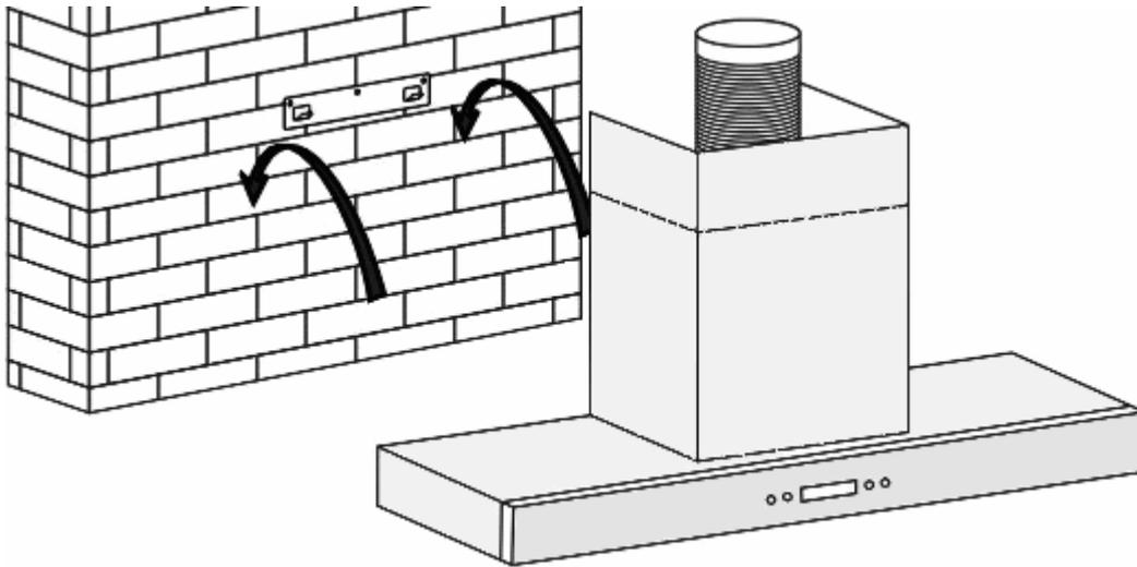
10. Secure the base of the hood with 2 x ST4x30mm anti-tilt screws to ensure unit is installed level, mounting holes for the screws are accessible via the fan motor chamber.
