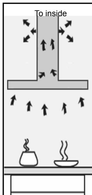
For air recirculation mode, charcoal filter (Optional Accessory) must be installed to eliminate cooking smells.
