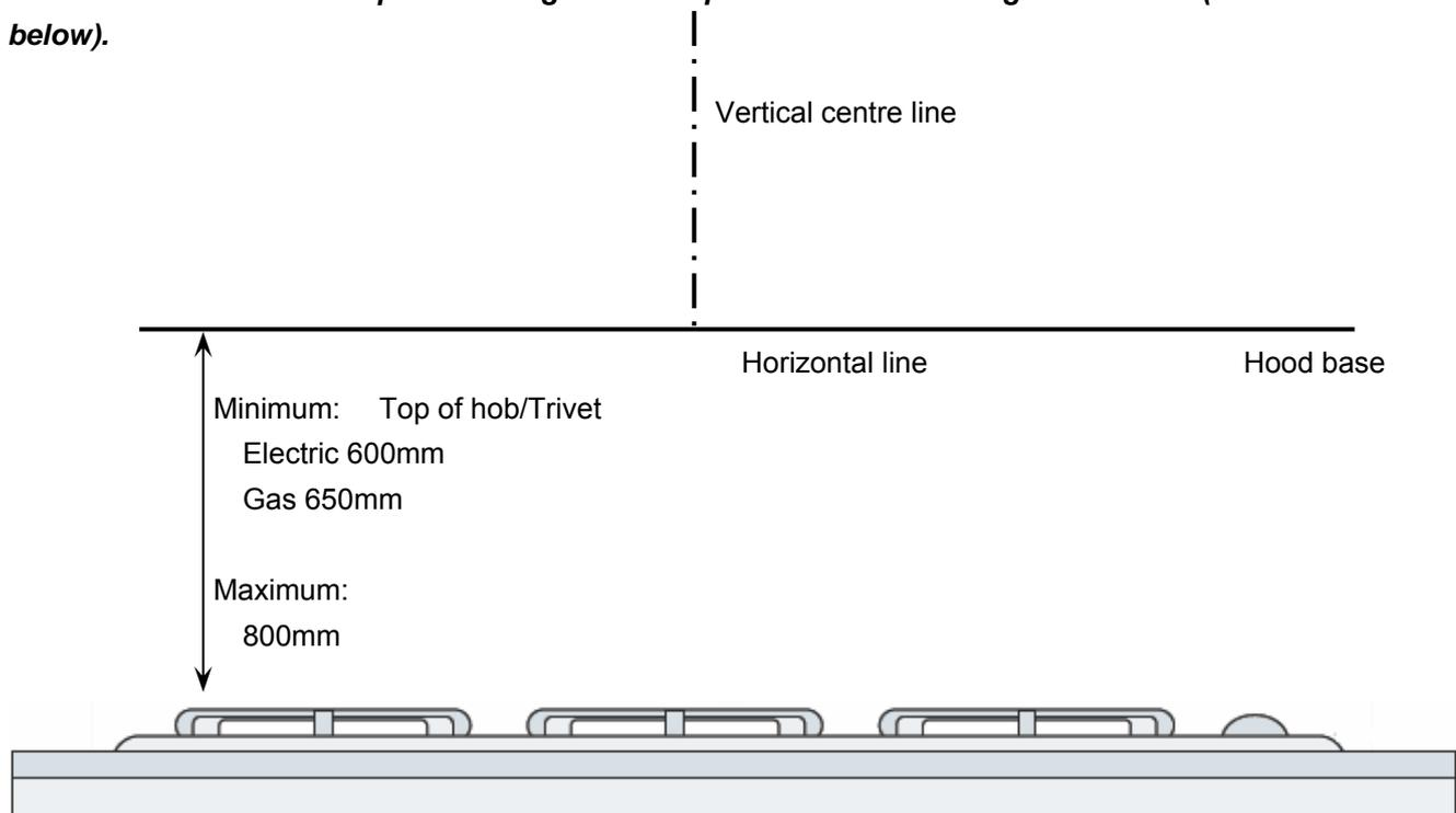
\*If the instructions of the hob specify a greater distance than the minimum above, then that shall be the minimum height for installation
