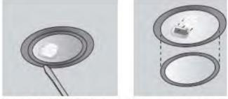
Using a small flat blade screwdriver remove the inner stainless steel ring to obtain access to the halogen globe.
