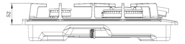
**NOTE:** On completion of the installation of the cooktop to the kitchen bench, the distance from benchtop surface to the highest part of any trivet is 46mm as shown in illustrations for model BG905X.
