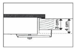
Then a particle board or similar heat baffle must be installed under the hob to prevent accidental touching of the underside surface.
