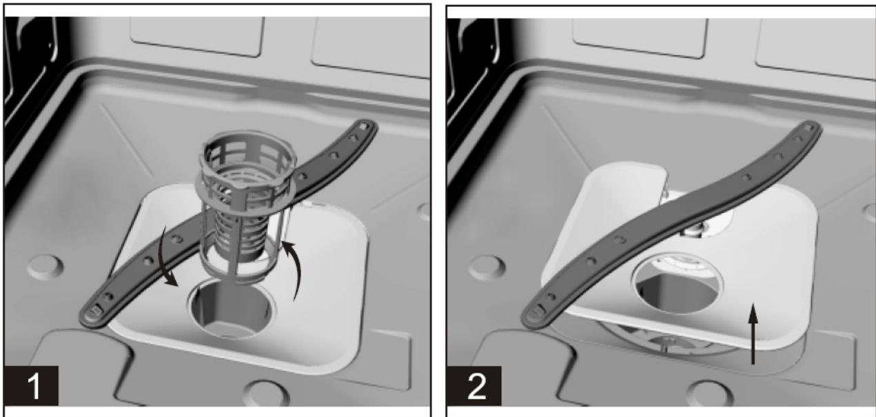
Then, reassemble the filter parts as shown in the figures below and reinsert the entire assembly in the dishwasher, positioning in its seat and pressing downward.
