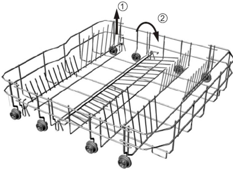
Folding racks consisting of two parts that are located on the lower basket which are designed to allow you place big items easier as pots, pans, etc. If needed, each part can be folded separately, or all of them can be folded for larger space. You can use folding racks by raising them upwards, or by folding.
