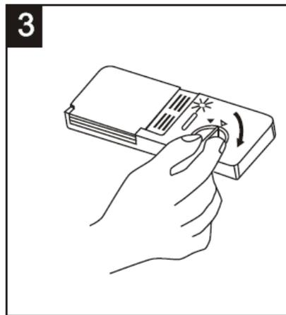
1. Open the dispenser, turn the cap to the "open" (left) arrow and lift it out.
