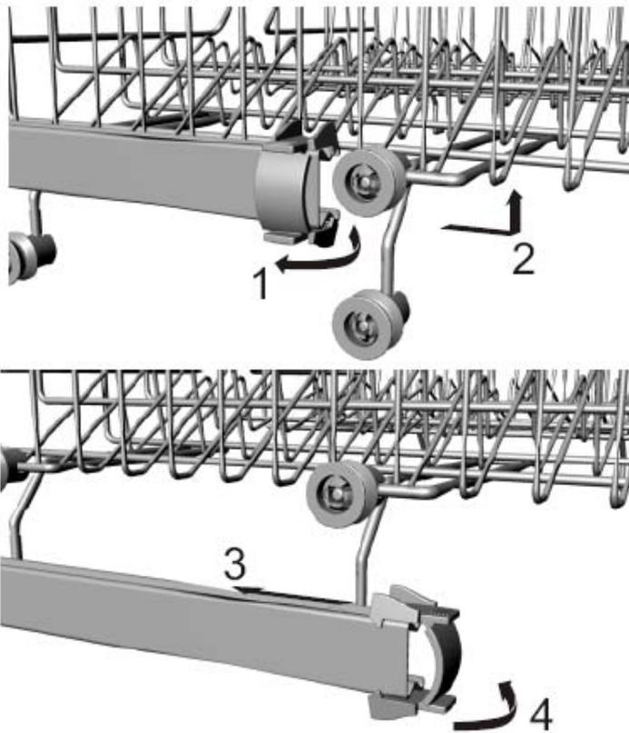
If needed, height of the upper basket can be adjusted to create more space for large utensils either in the upper basket or lower basket. The upper basket can be adjusted for height by putting wheels of different height into the rails. Long items, serving cutlery, salad servers or knives should be placed on the shelf so that they do not obstruct the rotation of the spray arms. The shelf can be folded back or removed when not be required for use.
