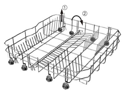
Folding racks consisting of two parts that are located on the lower basket which are designed to allow you place big items easier as pots, pans, etc. If needed, each part can be folded separately, or all of them can be folded for larger space. You can use folding racks by raising then upwards, or by folding.
