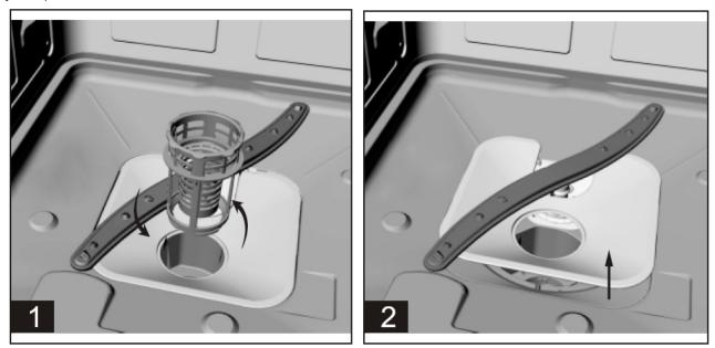
Then, reassemble the filter parts as shown in the figures below and reinsert the entire assembly in the dishwasher, positioning in its seat and pressing downward.
