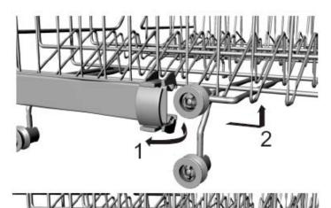
If needed, height of the upper basket can be adjusted to create more space for large utensils either in the upper basket or lower basket. The upper basket can be adjusted for height by putting wheels of different height into the rails. Long items, serving cutlery, salad servers or knives should be placed on the shelf so that they do not obstruct the rotation of the spray arms. The shelf can be folded back or removed when not be required for use.
