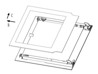
**Step 3:** Undo the screw on the clips "No.1" on the left and right doorframe.
