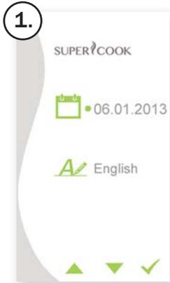
1. Use the ▼ ▲ buttons to switch between calendar and language and use the left and right rotary knob to adjust the settings.
