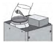
5. Remove the grease mesh filter and install active charcoal filter (Not Supplied) onto motor chamber refer below drawing.
