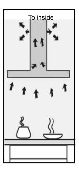
For air recirculation mode, charcoal filter is a must to eliminate cooking smells.
