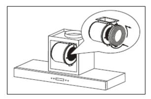
4) Hook the carbon filter over the pins that are located at the end of the motor.
