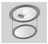
Using a small flat blade screwdriver remove the inner stainless steel ring to obt ain access to the halo gen globe.
