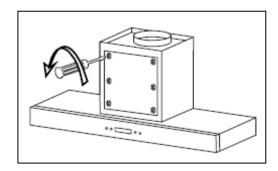
3) Once the motor access panel is removed, you will be able to see the motor.
