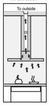
For air extraction mode, a ducting kit is required, the air is drawn in and cleaned by the grease filters and via the ducting must be directed to the outside atmosphere.
