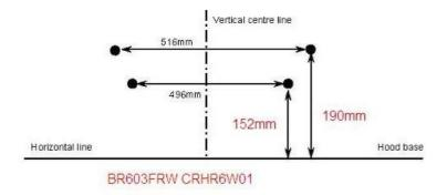
3 Hammer *dry wall anchor plugs* into holes. Insert 2pcs *Screw(ST4x30mm)* into the two lower holes(with distance to horizontal line 496mm) and fasten, they will be used to hang on the range hood.
