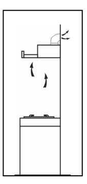
Ducting must be vented to outside atmosphere.
