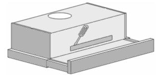
Remove mesh filters from the range hood then you will see the shifter, you can choose air exaction mode or air recirculation mode by turning the shifter to corresponding position.
