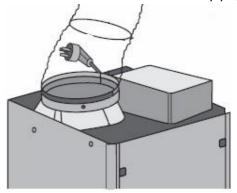
5. Remove grease mesh filter and install active charcoal filter onto motor chamber according to below drawing. \* If choose air extraction mode, please skip this step and jump to step 6 directly. if choose air recirculation
