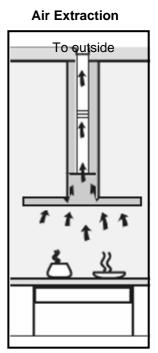
For air extraction mode, a ducting kit is required, the air is drawn in and cleaned by the grease filters and directed outside.
