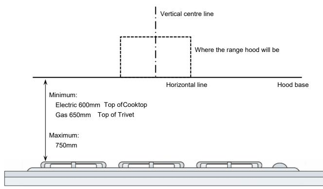
\*If the instructions of the hob specify a greater distance than the minimum above, then that shall be the minimum height for installation
