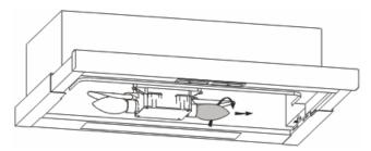
Remove two grease mesh filters, twist to remove bulb, whilst cool, and replace carefully with a new bulb. The range hood takes 2 x 40W incandescent bulbs. Important
