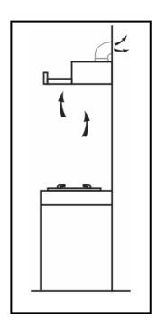
For this mode, a ducting kit is required, the air is drawn in and cleaned by the grease filters and directed outside.
