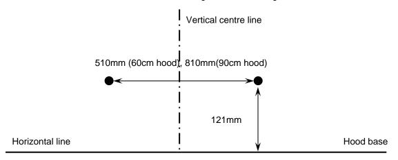
3. Hammer *dry wall anchor plugs* into holes. Insert 2pcs *Screw(ST4x30mm)* into the 2 holes(with distance to horizontal line 121mm) and fasten, they will be used to hang on the range hood.
