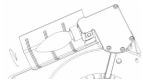
Remove two grease mesh filters, twist to remove bulb, whilst cool, and replace carefully with a new bulb. The range hood takes 1 x 28W incandescent bulbs.
