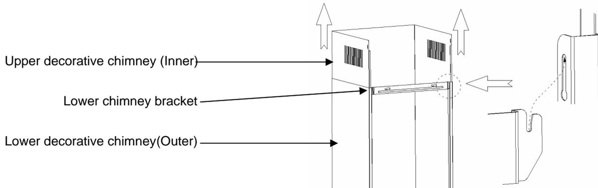
12. Determine position where *upper decorative chimney* maximum extent to, use 2pcs ST4x30mm screws to secure *the upper decorative chimney bracket* onto wall.
