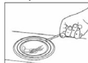
When handling globes hold with a cloth or gloves to ensure perspiration does not come in contact with the globe as this can reduce the life of the globe.
