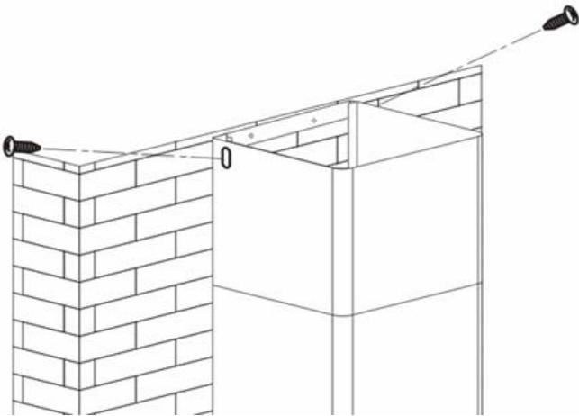
14. Remove all blue protective film on chimney and cooker hood, the installation is now finished.
