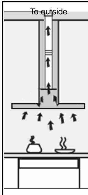
For air exaction mode, a ducting kit is required, the air is drawn in and cleaned by the grease filters and directed outside.
