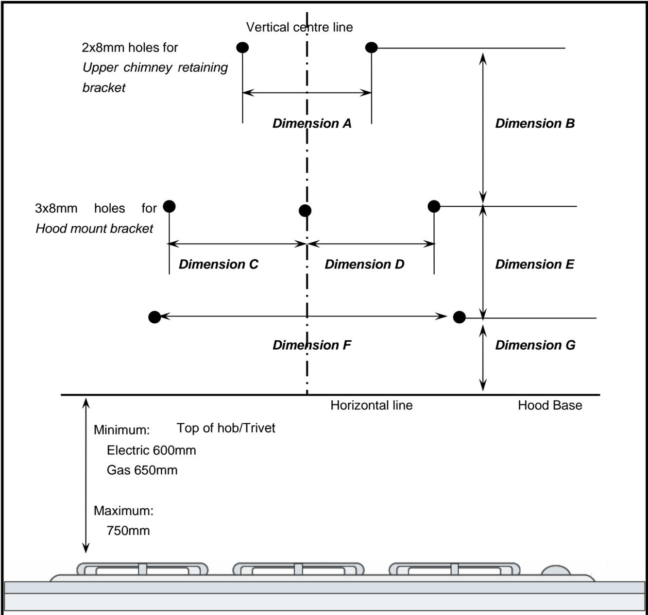
\*If the instructions of the hob specify a greater distance than the minimum above, then that shall be the minimum height for installation
