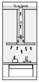
For air extraction mode, a ducting kit is required, the air is drawn in and cleaned by the grease filters and directed outside.
