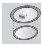
Using a small flat blade screwdriver remove the inner stainless steel ring to obtain access to the halogen globe.
