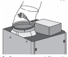
5. Remove *grease mesh filter* and install active charcoal filter onto motor chamber according to below drawing.
