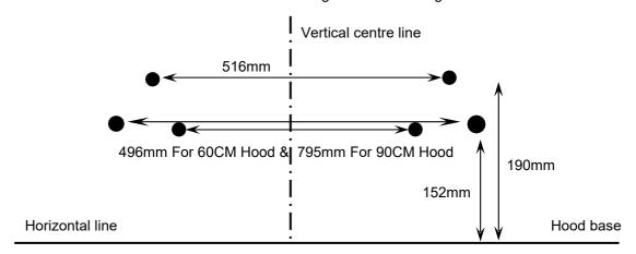
3 Hammer *dry wall anchor plugs* into holes. Insert 2pcs *Screw(ST4x30mm)* into the two lower holes(with distance to horizontal line 496mm 60cm & 795mm 90cm) and fasten, they will be used to hang on the range hood.
