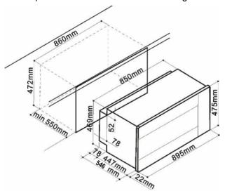
To provide adequate ventilation, there must be appropriate ventilation opening, the panel to which the oven is fitted should have a gap of at least 70 mm at the rear.
